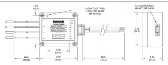
Standard enclosure. Note: Single channel systems use the x axis sensor connectors.
